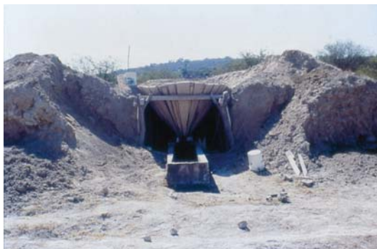
Salt Production in Mesoamerica. Fig. 2 This device, known as estiladera , is used for filtering the water from the springs through salty soil to obtain brine by leaching (© Eduardo Williams).
